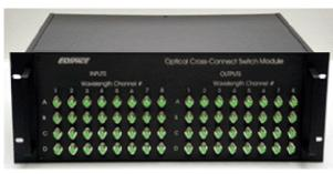
A 32 x 32 (4 paths, each with 8 wavelengths) optical cross-connect module
