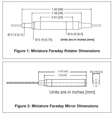
Miniature Faraday Rotator Package For 1300-1550 nm & 1064 nm
