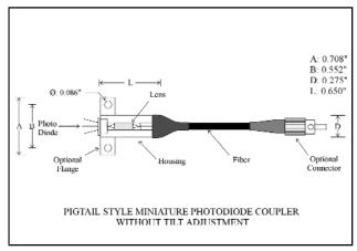
is adjusted until the maximum coupling efficiency is achieved. Typical coupling efficiency exceeds 80 percent for singlemode fibers, although this varies, depending on the fiber and photodiode characteristics. The tilt adjustment design is recommended for getting the best coupling efficiencies into very small surface area photodiodes.
