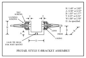
connectors, including NTT-FC, AT&T-ST, bare fiber adapters, etc. Typical insertion losses are 1.0 dB across a 60mm gap for connectorized versions, with backreflection levels typically -20 dB.
