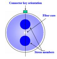
Slow axis align with connector key
